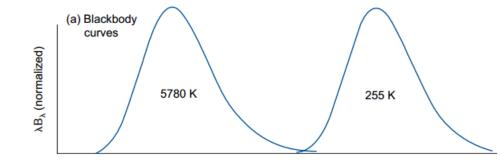
Since the Sun and the Earth are at very different temperatures, the emission spectra are almost completely separate.
