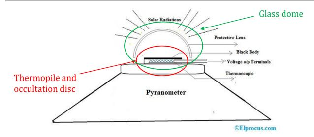
**Thermopile:** it uses a thermocouple used to notice dissimilarity in temperature between two surfaces. These are hot (labeled active) and cold (reference) accordingly. The labeled active surface is a black surface in flat shape and it is exposed to the atmosphere. The reference surface depends on the difficulty of the pyranometer because it changes from a second control thermopile to the covering of the pyranometer itself.
