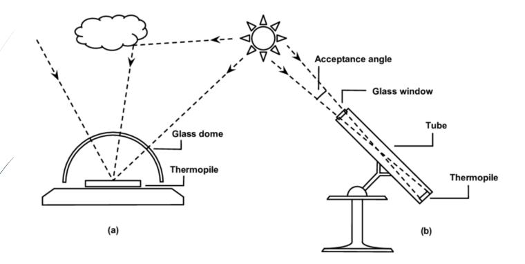
Pyranometer is used to measure diffused sun energy. **Pyrheliometer** is used to measure the sun's energy directly.
