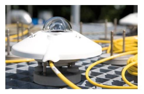
The <u>shape of the dome</u>, and the <u>refractive index</u> of the material, improves the response of the sensor when the sun is close to the horizon, 'bending' the incoming radiation beam.
