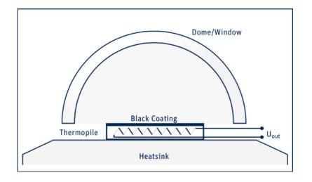
It is necessary to protect the black detector coating against external influences which may affect the measurement (precipitation, dirt, wind).
